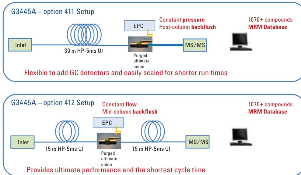
Figure 1. System configurations of Agilent GC/MS/MS Multiresidue Analyzers.
