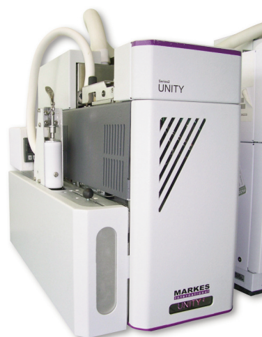
Figure 1. HS5-TD accessory (left) connects directly to the UNITY 2 TD instrument (right)
