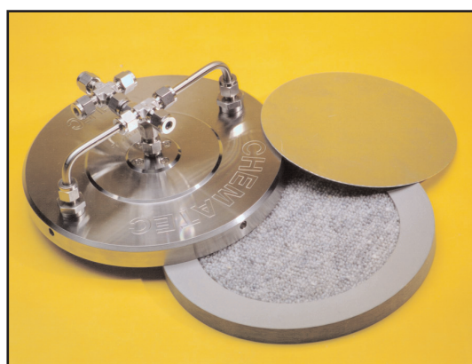
Figure 4: FLEC cell for sampling gaseous emissions from construction materials
