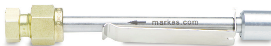
Figure 2: Axial diffusive sampler fitted with brass storage cap, pencil, and diffusion cap.
