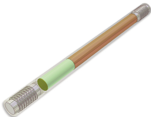
Figure 4: Schematic of SafeLok tube incorporating diffusion-locking inserts at both ends, shown here with two sorbent beds.
