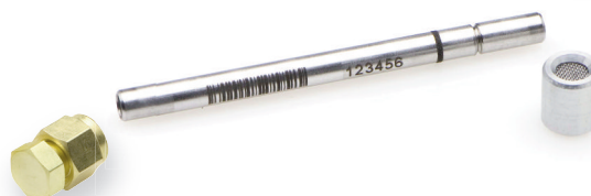
Figure 2: A sampling tube, brass cap and diffusion cap.
