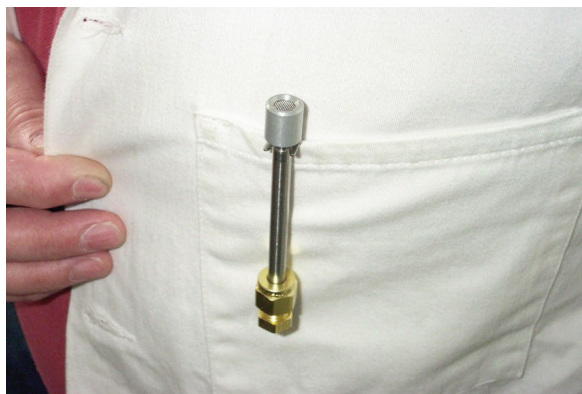
Figure 2: A thermal desorption sampling tube being used in diffusive (passive) mode, with the sampling end uppermost.
