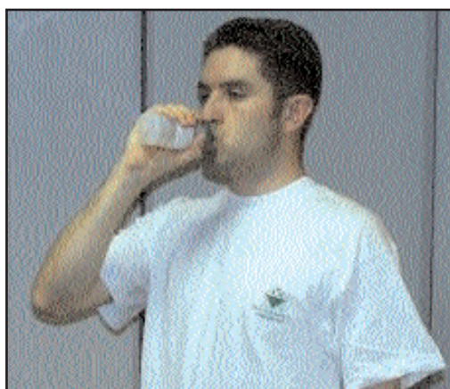
Figure 6: Monitoring biological exposure via alveolar air collected using the Bio-VOC breath sampler
