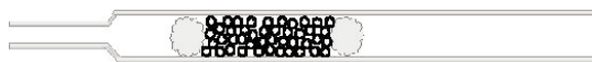
Figure 1: Schematic of sample loaded into a PTFE liner ready for insertion into an empty stainless steel tube.
