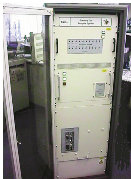
Figure 7: A 19" rack-mounted TD-MS system.
