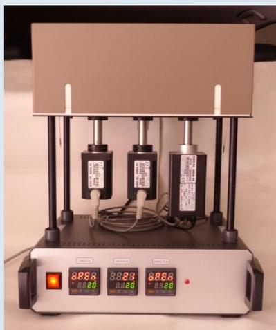
The SSI-16 Interface is an automatic multi sample loop Storage Sample Interface for coupling a TGA to a GC/MSD from any vendor.
