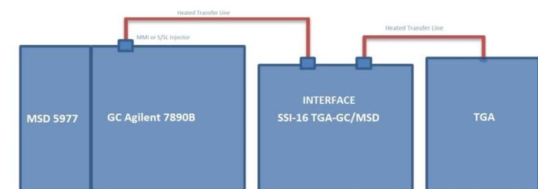
The ISS-16 is installed between TGA and GC. It requires 40 cm (W) of bench space.
