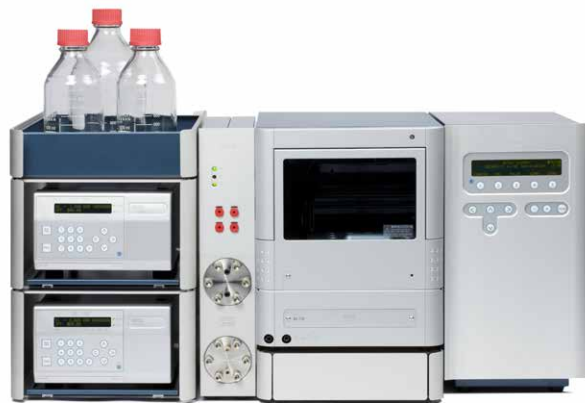
Figure 1: ALEXYS Aminoglycosides analyzer for Spectinomycin
