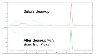
Figure 3. Comparison of the chromatograms of ammelide in fortified milk sample before and after clean-up with Bond Elut Plexa.
