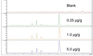
Figure 4. TIC of milk fortified with melamine and related compounds at low, mid, and high concentrations and blank extract.
