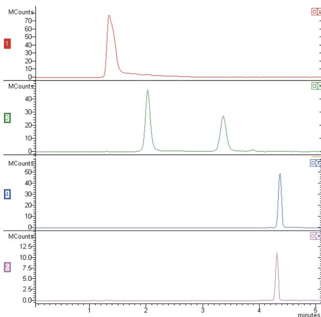
Figure 1 – Separation of all metabolites in a single 5 min run; from the top, Nicotine, Morphine, Estradiol, and Naphthol.
