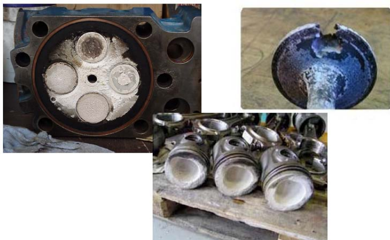
Figure 2: Defects on engine parts caused by silicon
