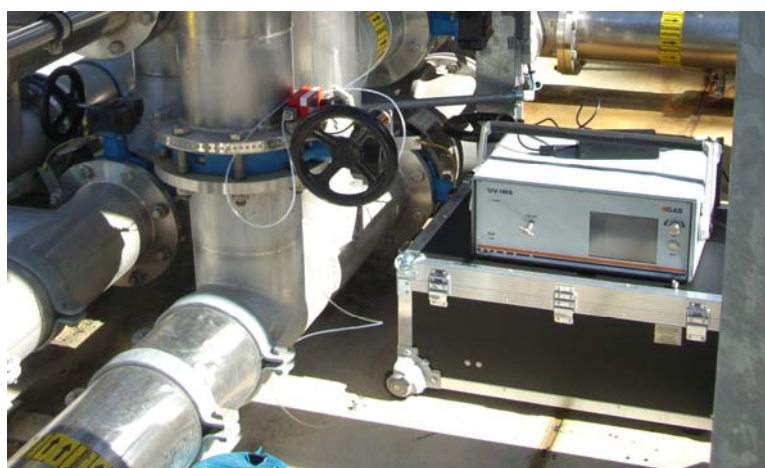
Figure 3: GC-IMS-SILOX on-site at biogas plant
