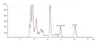
This overlay represents 10 samples prepared with the Agilent 7696A Sample Prep WorkBench. EPA method standards specify 0.1-5.0 vol% for benzene and 2-20 vol% for toluene
