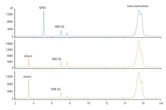
14 different ethers and alcohols from 0.1-15 wt% were detected. Samples were prepared with the Aqilent 7696A Sample Prep WorkBench.
