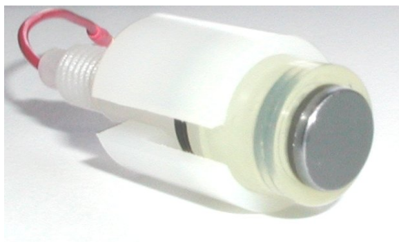
Fig. 9. Working electrode assembly with Magic Diamond electrode .
