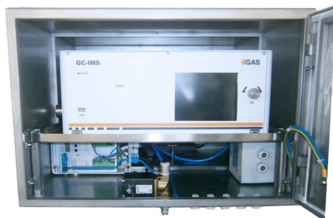
Figure 4: GC-IMS instrument for monitoring of TICs in chemical plants embedded into a pressurized enclosure system. The pressurized enclosure system ensures safety class Ex II 2 G Ex px II T4 (German Explosion Protection Ordinance).
