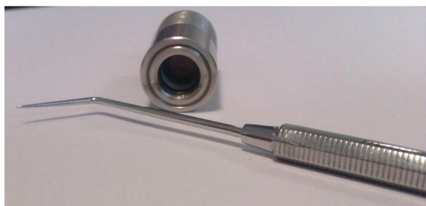
Figure 6: Back-pressure adapter with O-ring extraction tool.
