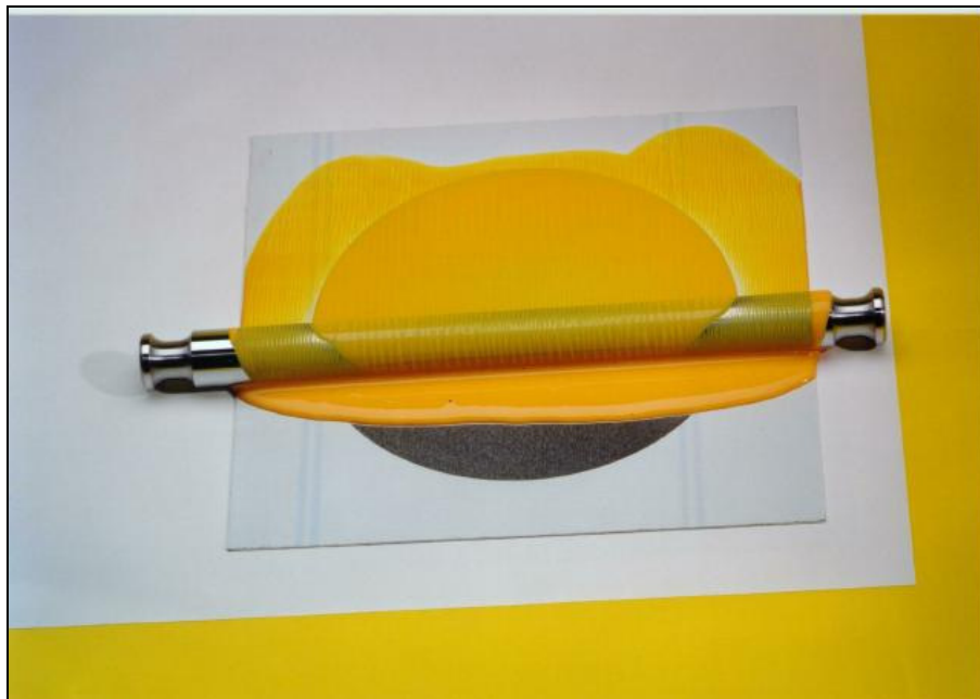
Figure 2. Application roller and test plate for paints and coatings
