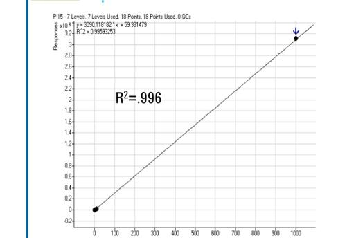
Figure G Calibration Curve for P-15 in HA 710 Zeptomoles/ $\mu$ L to 710 attomoles/ $\mu$ L
