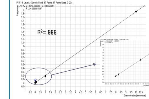
Figure F Calibration Curve 70 Zeptomoles/ $\mu$ L to 0.7 Picomoles/ $\mu$ L
