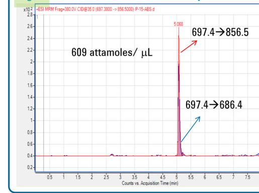
Figure D Reproducibility of three injections: 4% RSD, 140 attomoles on column
