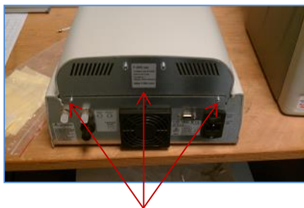
Remove the three bottom screws
