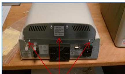
Remove the three bottom screws
