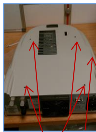
Remove the four screws
