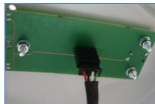
Disconnect the cable of the interface
