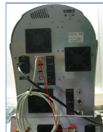
Connect the RS485 cable
