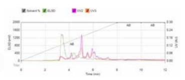
Purification of Neem Oil, 500mg on a REVELERIS® 40g silica cartridge (upper) and a REVELERIS® HP 40g silica cartridge (lower).
