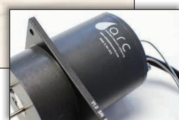
The Polyarc system has a catalytic microreactor that enhances new and existing gas chromatographs (GCs) with flame ionization detectors (FIDs) by converting all organic compounds to methane molecules prior to their detection by the FID. In doing so, the Polyarc system reduces the need to perform time-consuming calibrations by creating a uniform detector response for truly universal carbon detection.
