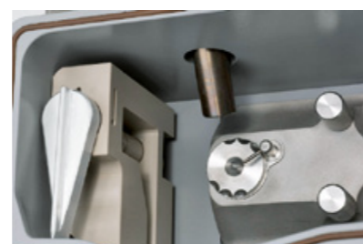
Detail of MSQ Plus with electrospray ionization (ESI) installed
