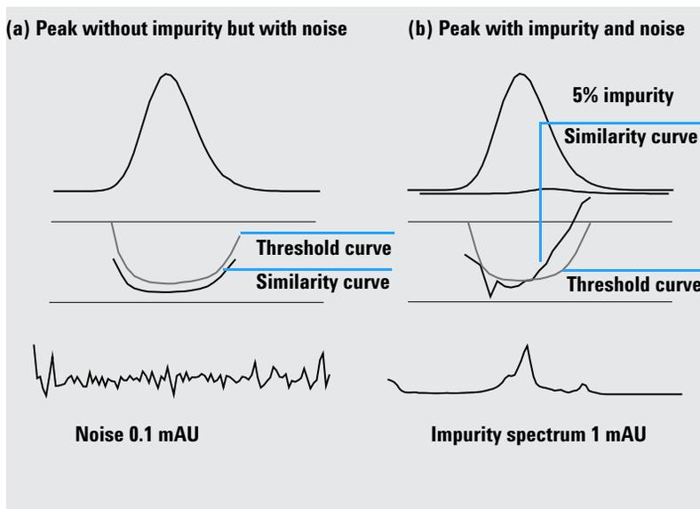
**Figure 8** Effect of Impurity and Noise on Similarity and Threshold Curves
