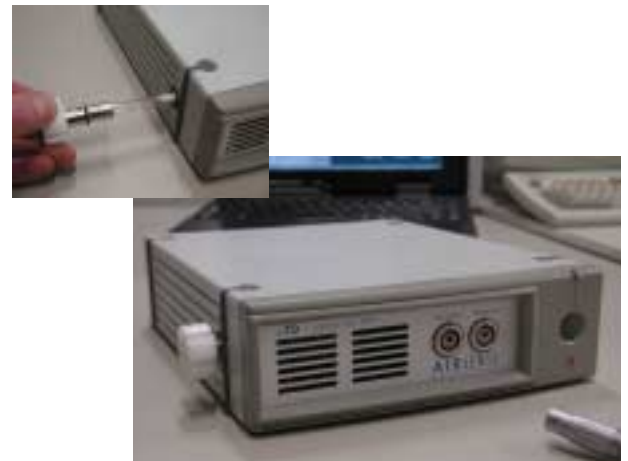
Fig.5: Specialized TTD unit ( \mu TD) optimized for operation with a Micro-GC
