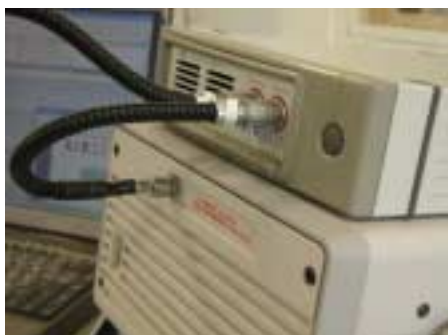
Fig.4: TTD unit Attached To Agilent Micro-GC
