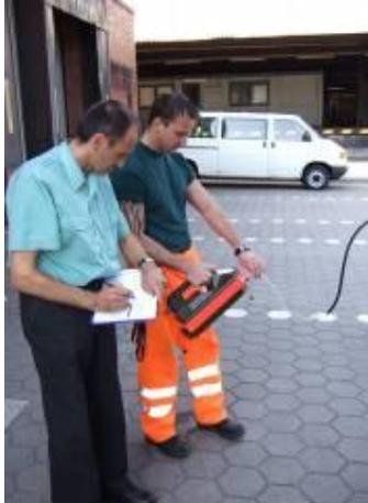
Bild 2: Analysis and protocol of the results shown by the GDA2. (Customs service, Hamburg)
