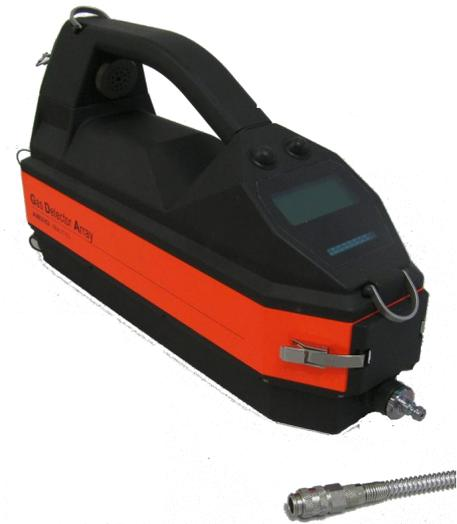
The GDA2 *Fumigation* is a portable detector which is operated directly at the container and able to respond within seconds if dangerous concentrations of hazard chemical substances can be found there or not.
