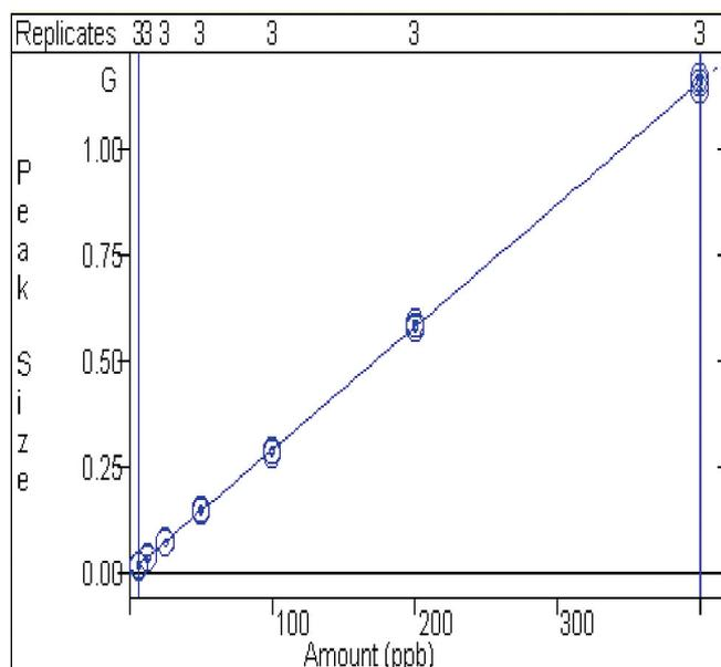
Figure 5 Calibration curve of nivalenol spiked in solvent.
