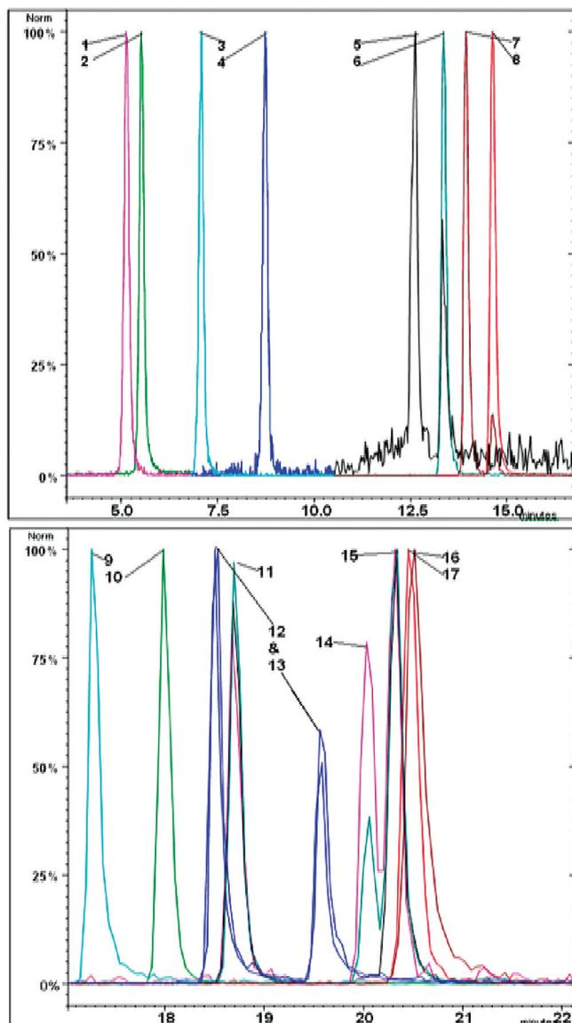
Fig 2 Normalized chromatograms of the 16 mycotoxins in the multi-component method. The numbered label on each chromatogram corresponds to the respective mycotoxins given in Table 3.
