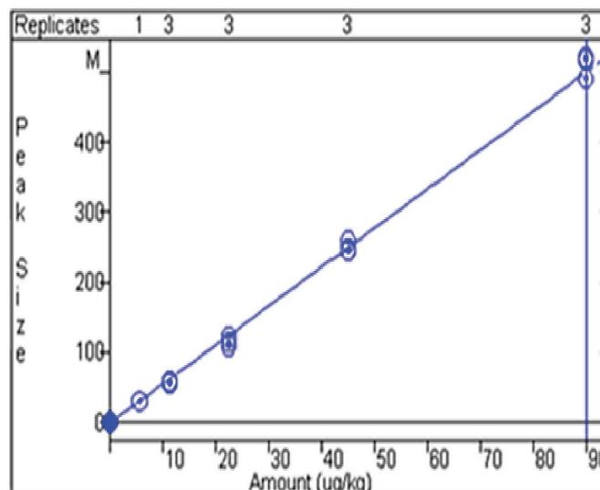
Figure 6 Calibration curve of  $\beta$ -zearalenol spiked in corn extract.
