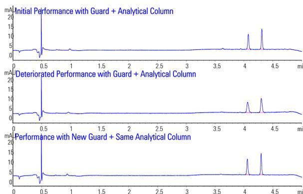
Chromatographically speaking, the dilute Similac sample causes the peaks to broaden and the pressure to increase, as proteins and particulates deposit at the head of the guard column and on the inlet frit. Replacing the old guard column with a new guard column restores performance back to its initial state.
