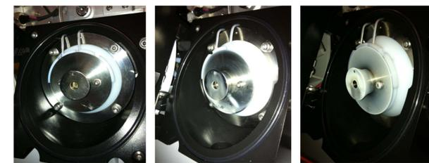
The clean LC/MS source (left) provides the most sensitive, reliable data. Ideally the cleanliness of the source is maintained to prevent contamination or interferences such as ion suppression.
