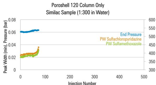
Installing a guard column prior to the analytical column preserves the lifetime of the more expensive analytical column. Below, 5 guard columns are sequentially changed out to show consistent performance over more than 400 injections with the same analytical column.
