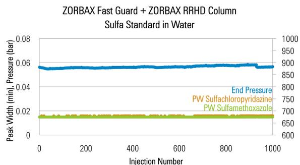
Chromatograms verify the consistent performance of the 2 analytes, sulfachloropyridazine and sulfamethoxazole, with no significant change in peak shape or pressure over the course of 1000 injections at 900 bar.
