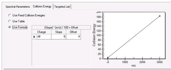
**Figure 32** Collision Energy tab showing calculated values
