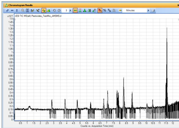
**Figure 33** Total ion chromatogram of the test mix run with auto MS/MS settings.
