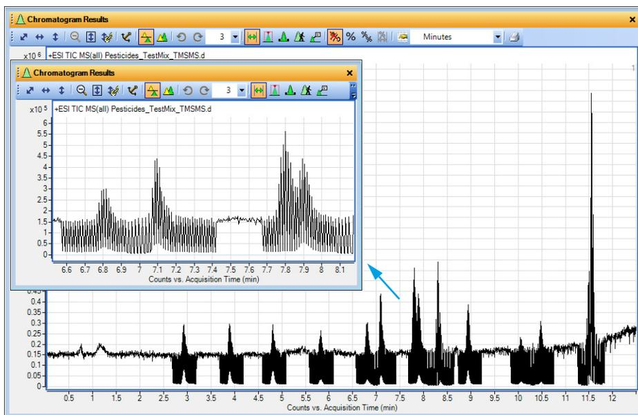
**Figure 19** Total ion chromatogram from a typical targeted MS/MS data shows sawtooth pattern from alternating MS and MS/MS scans.
