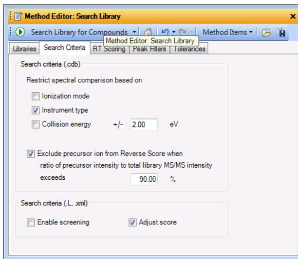
**Figure 40** Search Criteria tab with Collision energy check box cleared.
