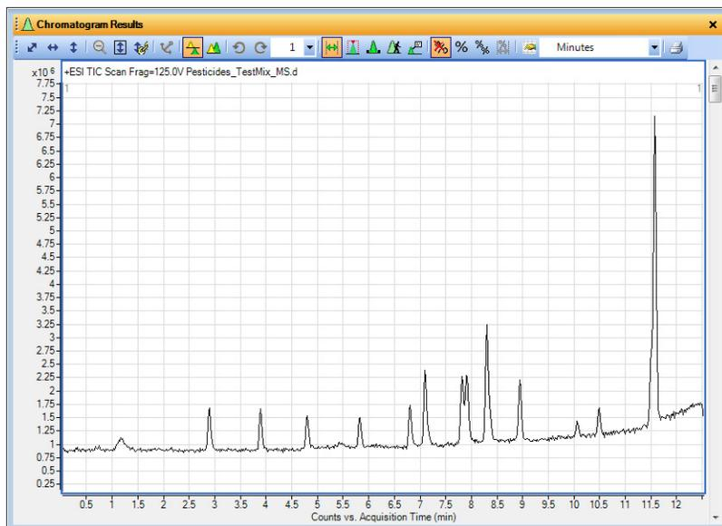
**Figure 7** Example Test Mix Total Ion Chromatogram
