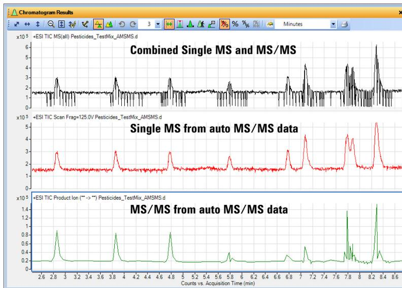
**Figure 36** The top chromatogram shows all of the data points for single-MS and MS/MS. Note that MS/MS data points have lower total signal because ions in a narrow mass range are isolated for fragmentation. The middle chromatogram shows the single-MS only and it is clear that the Q-TOF LC/MS is collecting mostly single-MS data. The bottom chromatogram is created by connecting all points where MS/MS spectra were acquired.
