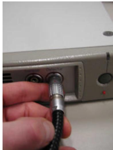
The transfer line is connected at the Micro GC by the 1/16" Swagelok nut. In order to avoid cold spots at the connection, it is important, that the thermal isolation of the transfer line ends close to the Swagelok nut.
