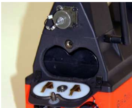
Fig. 54: Battery compartment open
