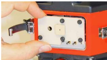
Fig. 11: Retire la tapa
