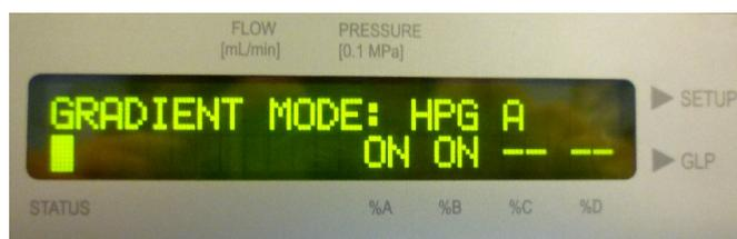
Fig. 17. Pump display when gradient mode for 2 pumps (HPG A and HPG B) is properly set. The first pump was configured as HPG A and both channels indicating %A and %B are ON.
