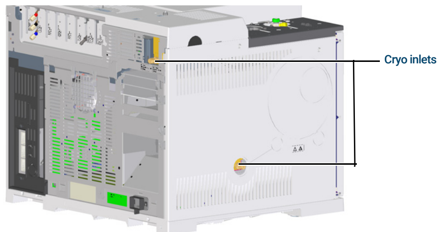
Figure 13. Location of cryogenic cooling valve
