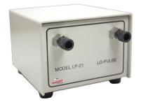
The noise level in the detector resulting from pump pulsations can significantly affect precision in qualification and the detection limit of trace components. The LO-Pulse™ pulse damper smooths pump pulsations and maintains constant flow in flow sensitive detectors.
