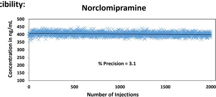
Repeatability evaluation using >2000 sequential injections of Norclomipramine
