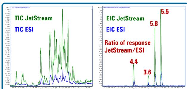
For capillary flow LC, a new AJS source was used with extended shielding of the nebulizer. This modification allows AJS to be used effectively at lower flow rates with a microflow nebulizer. This source gave a significant improvement in sensitivity compared to the ESI source (right).
