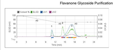
Column: Reveleris® Amino 40g flash cartridges Flow Rate: 40mL/min
