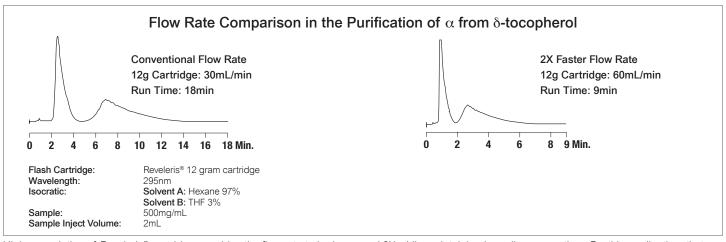
Higher resolution of Reveleris® cartridges enables the flow rate to be increased 2X while maintaining base-line separation. For this application, that results in over a 40% time savings per run.
