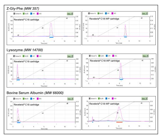
The Reveleris<sup>®</sup> C18-WP flash cartridges can be used to purify a wide range of molecular weight components, approaching 70,000 Daltons. The smaller particle size media increases resolution and makes the purification of complex large molecule mixtures more efficient.
