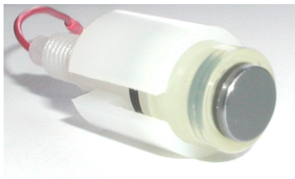
Fig. 12. Working electrode assembly with Magic Diamond electrode .
