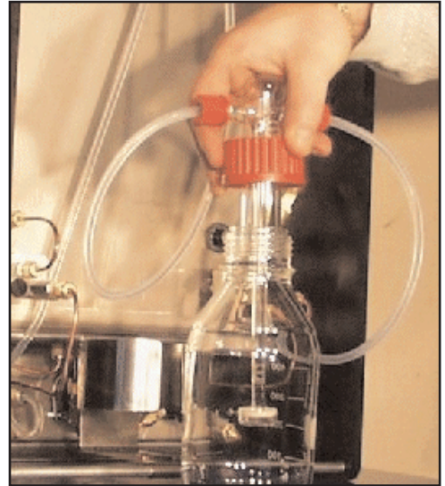
Figures 5 & 6 Removing the humidifier bottle
