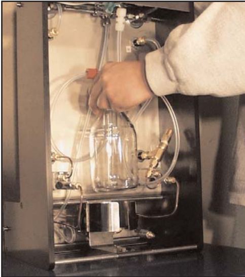
Figures 5 & 6 Removing the humidifier bottle
