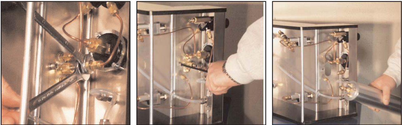
Figure 12, 13 & 14. Replacing the charcoal filter assembly
