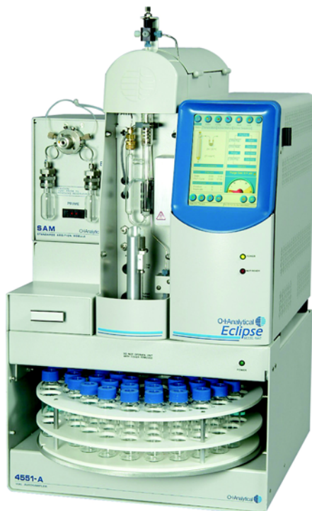
Figure 1. OI Analytical Eclipse 4660 P&T Sample Concentrator with Model 4551A Water Vial Autosampler and Standard Addition Module (SAM)
