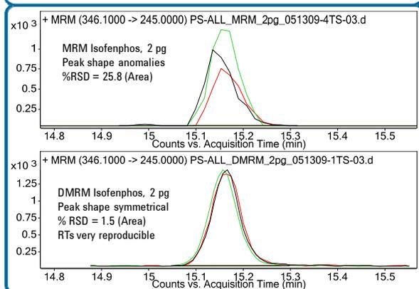
300 pesticides were analyzed in replicates of 3 at the 2 pg, 10 pg and 100 pg levels. For TS-MRM, mean %RSDs (area) were 13.4, 7.4 and 2.8 respectively. For DMRM, the results were 4.9, 2.3, and 1.3 respectively.
