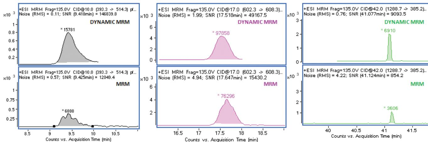
Figure 2. Comparison of peak symmetry obtained in MRM and DMRM.
