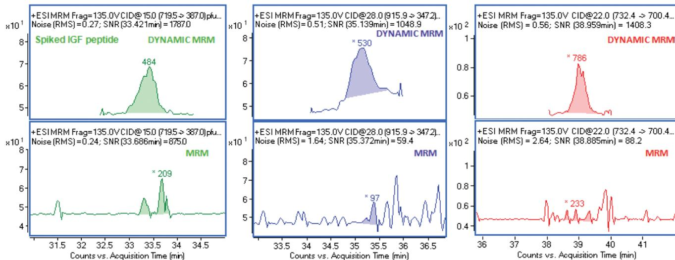
Figure 1. Examples of transitions demonstrating substantial sensitivity enhancement with DMRM.
