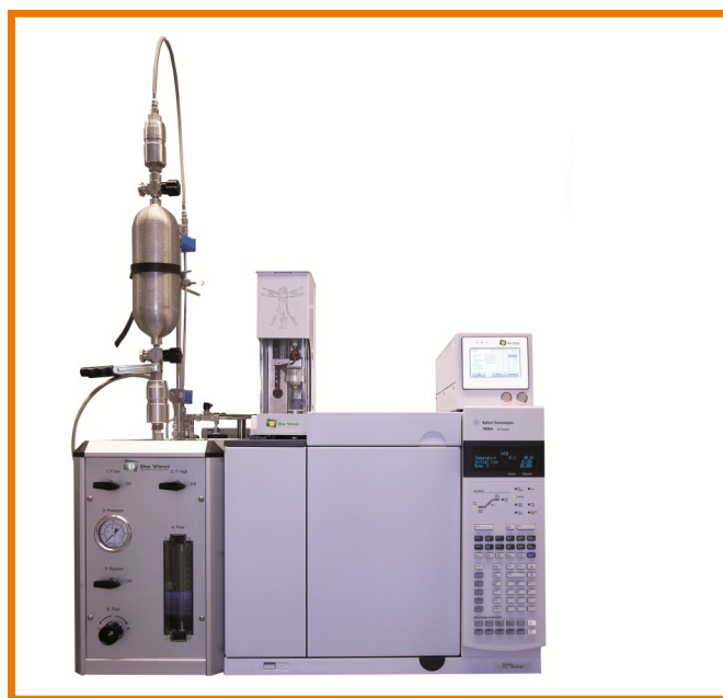
Figure One: the DVLS Liquefied Gas Injector
