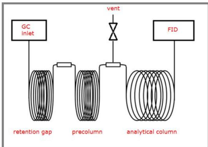
Figure Two: Typical Column Configuration for residue analysis using the LGI
