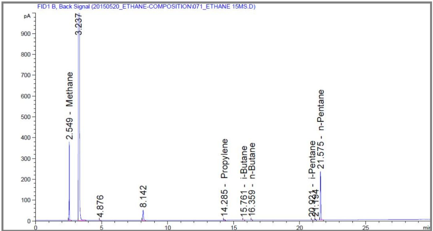
Figure Four: Chromatogram of the LGI analysis of light hydrocarbons of liquid Ethane
