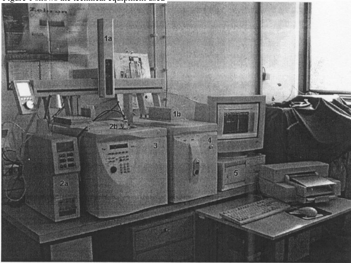
Figure 1: technical device consisting of 1a: automatic sampler (ATAS); 1b: sample rack with vials; 2a: control element of the thermodesorption-unit; 2b: thermodesorber; 3: GC (Finnigan); 4: MS (Finnigan); 5: Computer including GC-MS software
