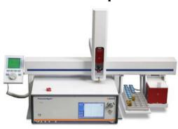
Detection of traces of VOCs in the headspace of solids & liquids in food/beverages
