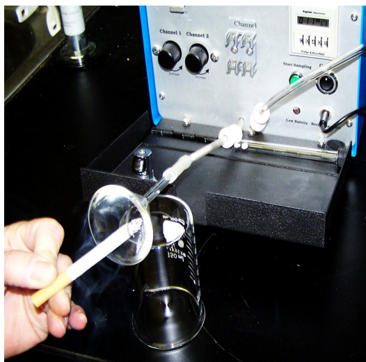
Figure 1. X-1067 Sampler set up to collect cigarette smoke
