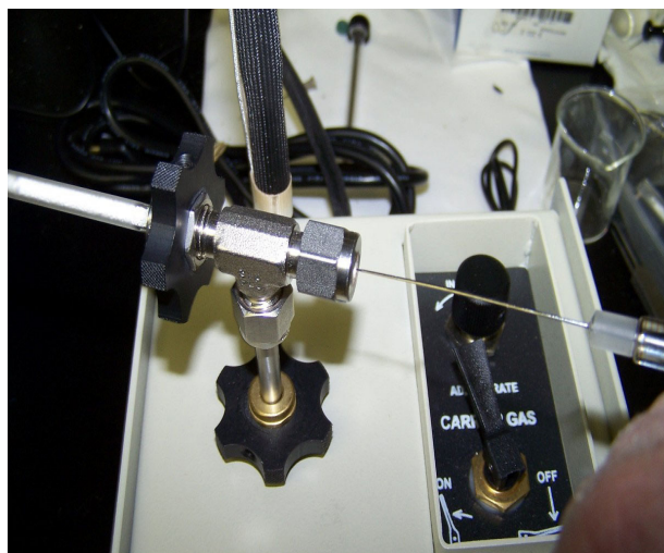
Figure 3. PFPH being spiked on a 3-bed sorbent tube using a CDS Tube Conditioner
